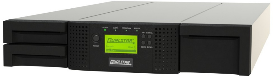
Entry-Level LTO Tape Library designed for SMB and distributed environments.
