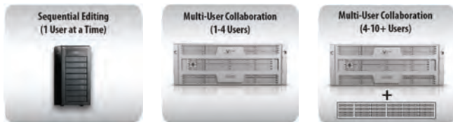
*Pegasus2: 1 user can write on a file at a time, multiple users can read. VTrak A-Class: Multiple users can write to the same file for true collaboration.
